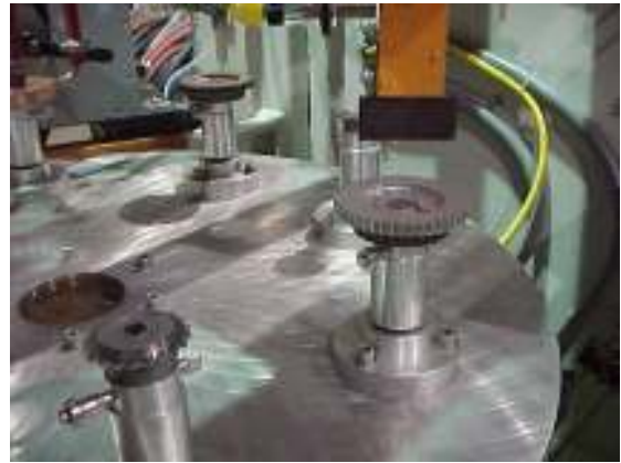
Profile gage to qualify part position (Position 2)
