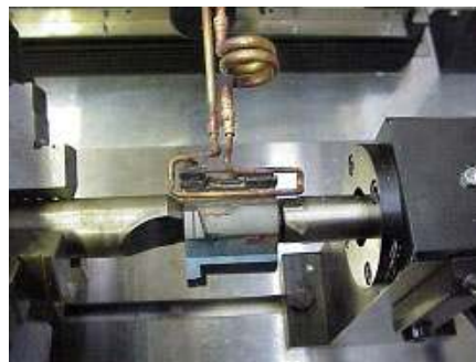
Three jaw chuck and tailstock holding part for brazing.
