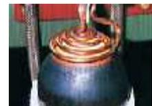
**Pre-forming heating of gas bottle bottom (thyristors inverter of 100 kW - 10 kHz).**
