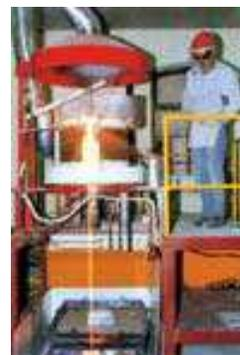
**Direct coil fusion of glass in a skull crucible (M.O.S. transistors generator of 100 kW - 200 kHz).**
