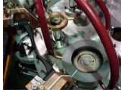
**High speed induction heating equipment processing 1200 parts/hour using the Accelerated Austenitizing™ process.**
