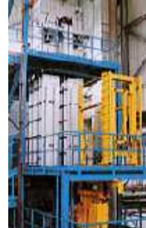
**Induction with sealed hydrogen unit for the re-heating of strips before galvanization (2 thyristors inverters of 1,500 kW - 6 kHz.).**
