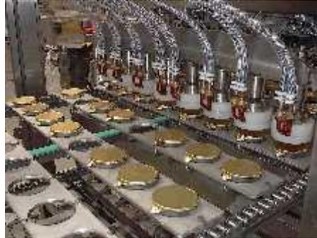
**Simultaneous heating of eight covers in 1 second using a 25kW/50kHz power supply with indexing conveyor.**
