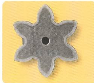
Fig 3 Image of a tooth hardened using the simultaneous dual-frequency (10 kHz and 120 kHz) method. Root circle diameter: 10 mm (0.40 in), tooth tip diameter: 20 mm (0.785 in).
