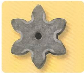
Fig 1 Image of the root of the tooth hardened using a medium frequency (10 kHz). Root-circle diameter: 10mm (0.40in); tooth-tip diameter: 20mm (0.785 in).
