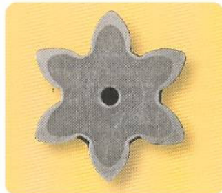
Fig 2 Image of the root of the tooth hardened using a high frequency (120 kHz). Root-circle diameter: 10 mm (0.40 in); tooth-tip diameter: 20 mm (0.785 in).
