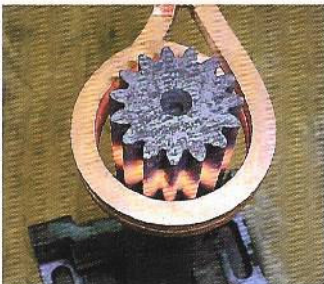
Simultaneous dual frequency applied to a single inductor. Plot shows coil voltage wave shape of medium frequency with superimposed high frequency and 70% medium frequency. Photo shows uniform heating of gear profile.
