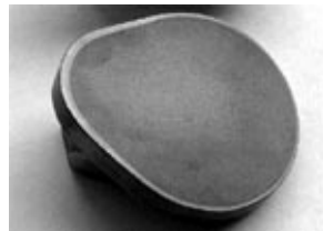
Cam lobe section of camshaft using our Accelerated Austenitizing™ process
