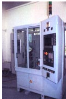
Vertical Scanner with PLC and integral quench system.
