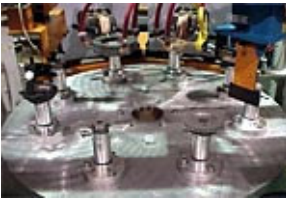
Dial table for processing production or pre-production parts.
