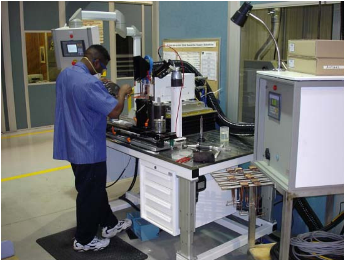
Complete system in operation for cutter carbide insert brazing.
